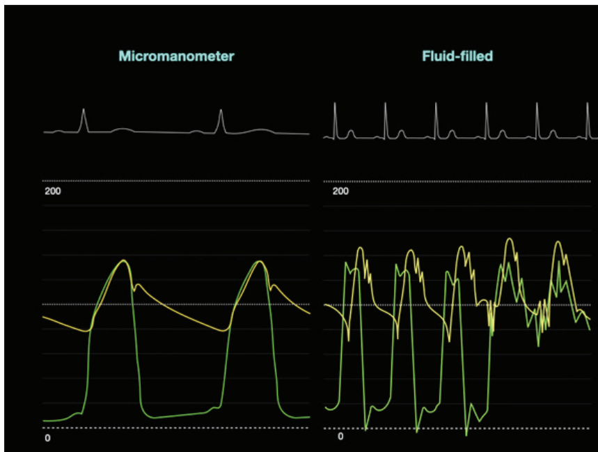
Figure 1. Simultaneous left ventricular and aortic pressure measurements using high-fidelity micromanometric catheters on the left, and simultaneous measurements of left ventricular pressure during a pullback into the aorta and femoral artery using fluid-filled catheters on the right.
